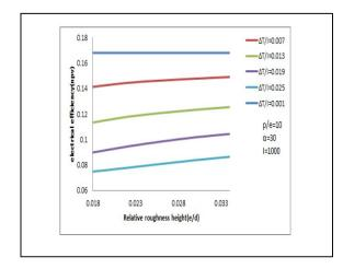
The larger values of this ratio are seen to correspond to higher values of temperature rise parameters, the lower values of temperature rise represent very high flow rate where the effect of roughness almost vanishes because of relatively high heat transfer coefficient even with smooth absorber plate and under such condition, the heat transfer coefficient (as also the friction factor) become independent of surface condition
